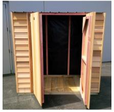
Step 25: Using 40mm screws, screw padbolt as shown, to the edge of the Left hand door ensuring padbolt will protrude at least 10mm into the floor when in locked position.
